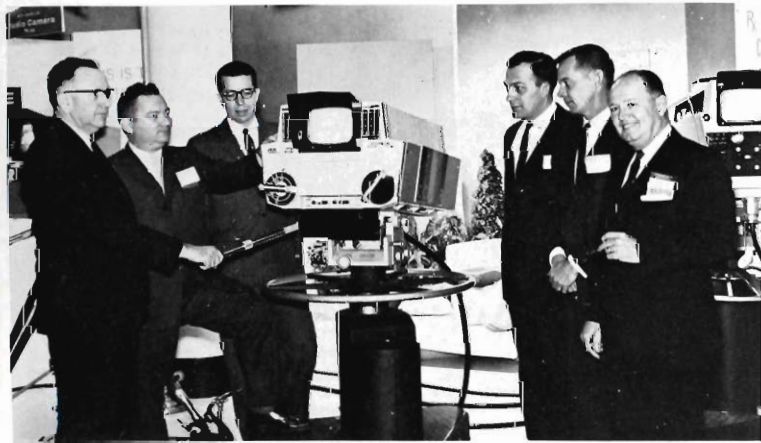
SOMETHING IN COMMON . . . both the cameras shown here—TK-42 for color, TK-60 for black-and-white—employ 4½-inch image orthicon for maximum picture detail. This big tube also provides finest pictures of color shows when viewed on monochrome receivers.
