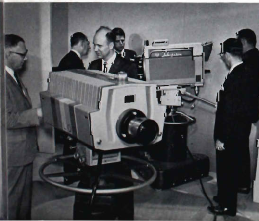
SOMETHING IN COMMON . . . both the cameras shown here—TK-42 for color, TK-60 for black-and-white—employ 4½-inch image orthicon for maximum picture detail. This big tube also provides finest pictures of color shows when viewed on monochrome receivers.
